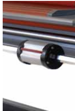
Auto grips to secure film cores to feed and wind up rollers
